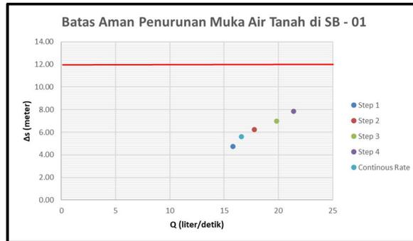
**Gambar 11.** Kriteria Aman Penurunan Muka Airtanah SB-01
